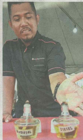
Uni10 Energy operations supervisor Yahirwan Yahya shows the difference between biodiesel made from recycled cooking oil (left) and fossil diesel (right) in a burning demo. The fossil diesel gives off more black smoke.
