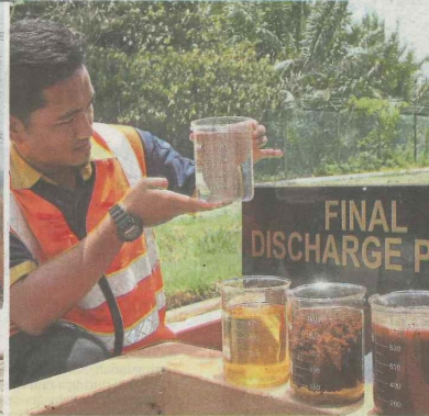
An employee Saiful Affandi Abdul Rani checking the water clarity and purity after going through the leachate treatment plant at the Jeram landfill.
